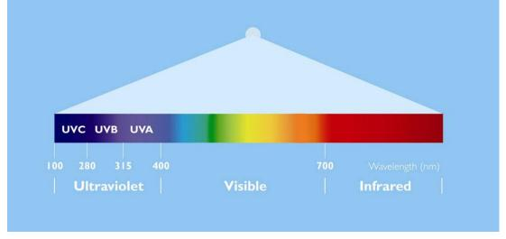
UVC radiation is known to break the DNA of bacteria, viruses and spores. As a result, they are rendered harmless.
